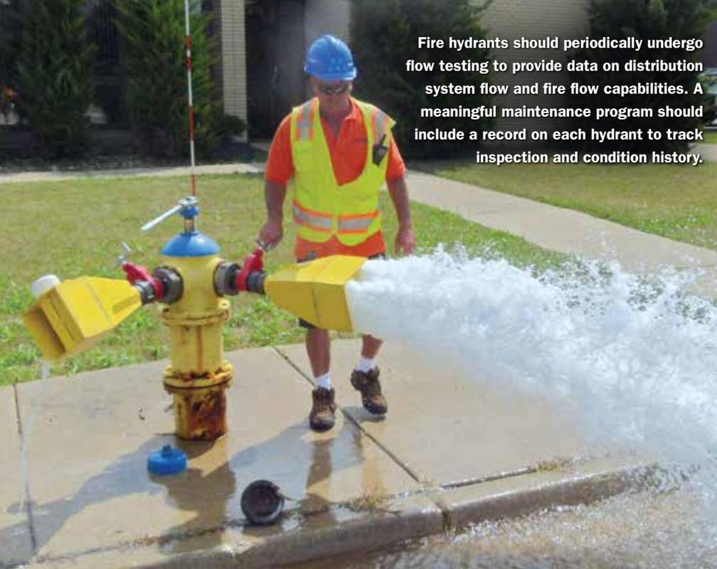
Fire hydrants should periodically undergo flow testing to provide data on distribution system flow and fire flow capabilities. A meaningful maintenance program should include a record on each hydrant to track inspection and condition history.
